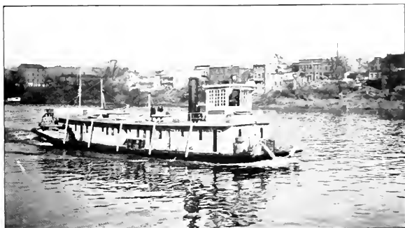
Diesel-electric shallow draft river tug J. B. Bantz, built by the Charles Ward Engineering Works, at Charleston, West Virginia, for the U. S. Engineers. We shall publish full description and drawings of this boat in a forthcoming issue.
